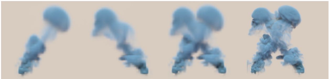
Fig. 4.4.11. Tracking the combination of two rising plumes. From left to right: A first low-resolution plume of smoke rising towards the top right corner, a second plume of smoke rising towards the top left corner, the result of the combination (by density summation) of the two previous simulations, and a tracked simulation generated using our method.
