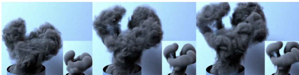
Fig. 2.5.9. Coarse smoke simulation and corresponding high-resolution smoke synthesized using the method of Chu and Thuerey [23] at three different times.
