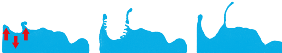
Fig. 2.2.9. Sculpting a liquid simulation using the approach from Stuyck and Dutré [119]. From left to right: An initial liquid simulation at a user-defined frame as well as user intents represented with red arrows, a sculpted keyframe after relaxation, the resulting liquid controlled to match the relaxed keyframe.
