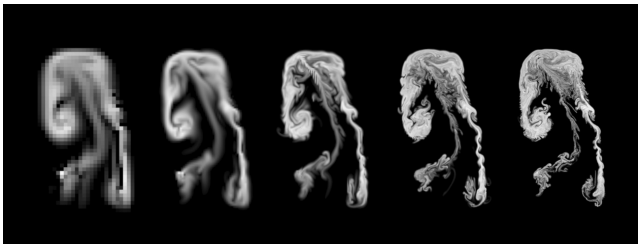
Fig. 5 2D rising plume. Left to right: guide ( 32\times 48 ), tracked 2\times , 4\times , 8\times , and 16\times . The larger the upresolution factor, the finer the added simulated details.
